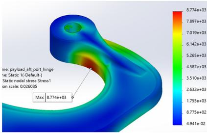
In finite element analysis on 3D printed polycarbonate hinges a weak link was identified at the base of the hinges where the hinge pin connects to the payload bed. This pivot point was analyzed for stresses exhibited in the event that the doors needed to be used to lift and flip the entire payload into the correct orientation, which would put extra stress on the hinges.
