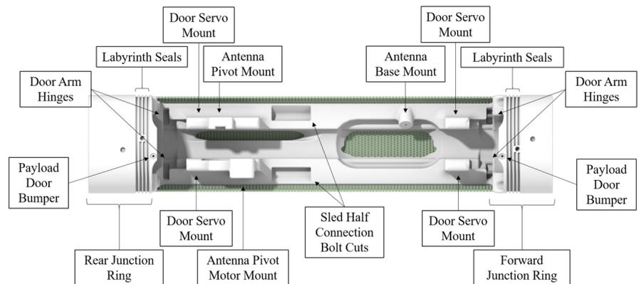
The freedom of design that comes with building a metal part layer-by-layer allowed the team to include complex design features into the hinges with ease.
