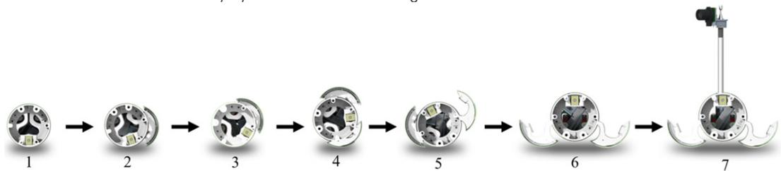
The payload mission of the 49er rocket *Fidem ad Finem* was to autonomously deploy, flipping the rocket if necessary, and receive radio frequency signals to command an onboard camera system and complete a series of tasks.
